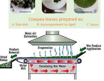
Figure 1: Mechanism of Refractance window drying ©mtcapra.com
